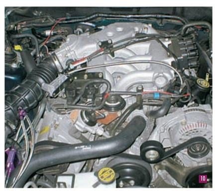
10. Follow the simple instructions provided with the ZEX kit to program the NMU and allow it to "learn" the vehicle's TPS voltage curve. Once this is done, the system is ready for use and will activate at wide-open throttle. With the ZEX installation complete, double check all of the fittings and connections.
