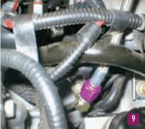
nitrous nozzle which ensures complete atomization of the nitrous/fuel mixture to develop maximum power and eliminate the risk of having the fuel puddle (which can lead to engine-damaging backfires).
