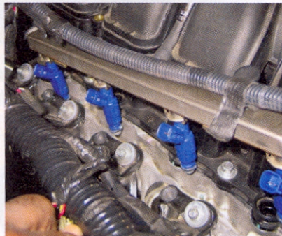
▲ We mentioned fuel volume being an integral part of performance/engine upgrades for late-model, EFI Mustangs. Turbonetics provides new 39-lb/hr fuel injectors with each kit, a set of eight Autolite HT0 (colder heat-range) spark plugs, and the all-important PCM calibration (uploaded via a DiabloSport Predator handheld flash tuner prior to hitting the dyno) that keeps combustion and evaporative emissions within CARB's accepted parameters, despite higher fuel flow.
