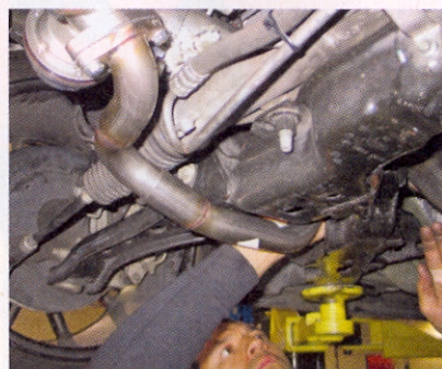
▲ This wastegate tubing tucks closely below the passenger-side A-arm and into the turbo system's exhaust tube. All of the stainless-steel/hot-side and aluminum/cold-side plumbing in Turbonetic's system is fully TIG welded. The system is designed with completely slip-fit pipes that are secured with 2.5-inch band clamps.
