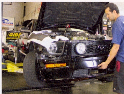
▲ Ricardo Topete of GTR High Performance in Rancho Cucamonga, California, performed the installation for us, which starts with securing the Mustang on a twin-post hoist, removing the battery completely, and then taking off the Pony's front bumper cover.
