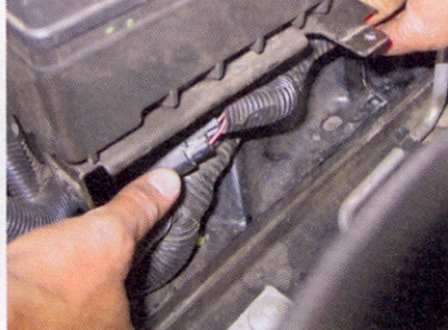
▲ The PCM is briefly removed to facilitate tucking the main engine harness into a pocket of space along the inside of the passenger-side fender. Having the wires out of the way eases positioning the turbo kit's 3-inch downpipe a bit. An air-conditioning line also is bent below the radiator at this time, for sufficient up-pipe clearance.
