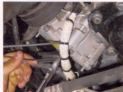
▲ Since the downpipe (the turbo's main hot-side tube) runs next to and below the passenger side of the engine, all wiring in those areas (starter, crank sensor, and so on) must be relocated or protected with tubing wrap. Wrapping wires and tubes is a tedious process, but it prevents damage to wiring due to extreme heat from the exhaust.
