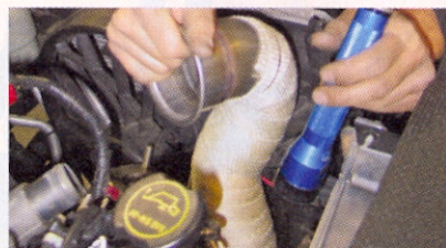
▲ Positioning the downpipe is a trial-and-error affair, as the 3-inch tube must be wrangled spot-on through a tight passageway between the engine and chassis. Notice the lip incorporated in the end of the pipe. Turbonetics includes a V-band clamp with the kit, which is used to secure the tube to the turbo's exhaust housing.
