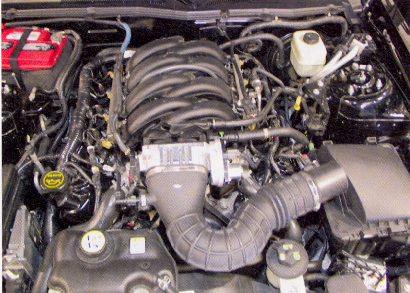
▲ Our '06 test Pony's bone-stock, 4.6-liter Three-Valve engine laid down a paltry 272.94 horses and 298.16 lb-ft of torque at the rear wheels in baseline tests. Turbonetics' 9-psi system should bring those numbers up considerably. We'll see when we get this baby on GTR High Performance's Dynojet chassis dyno.
