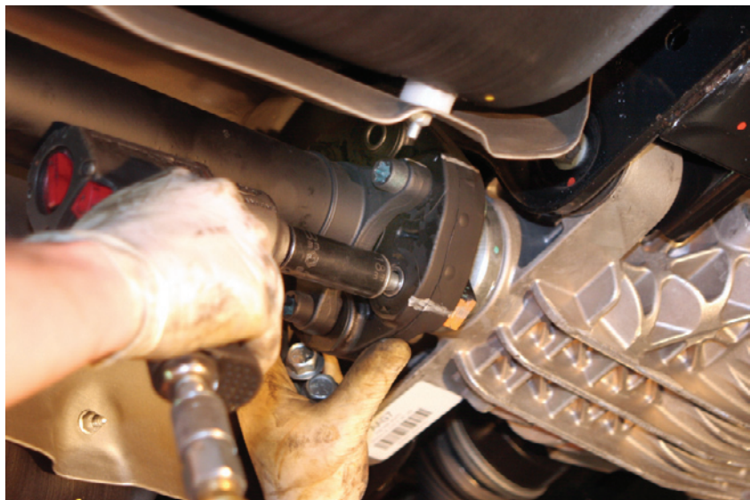
The driveshaft was marked (so it could go back into the same position) and then unbolted from the differential.
