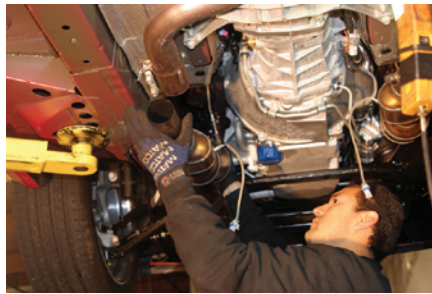
Ricardo Topete of GTR High Performance began by unbolting the exhaust clamps at the rear of the catalytic converter pipes.
