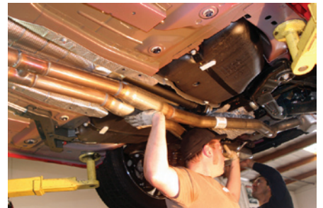
Removing the two hangers over the mufflers allows the exhaust to come out in one piece.
