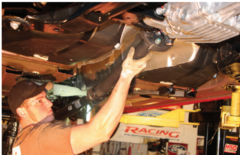
Once the driveshaft was unbolted from the front transmission output shaft, it could be removed and set aside.
