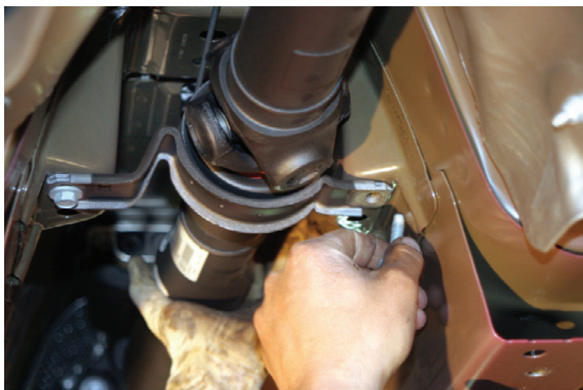
A center carrier bearing was also unbolted from the chassis.
