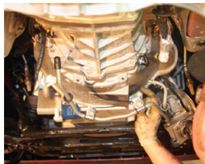
The coolant lines and wiring harness must be unplugged and removed from the transmission.
