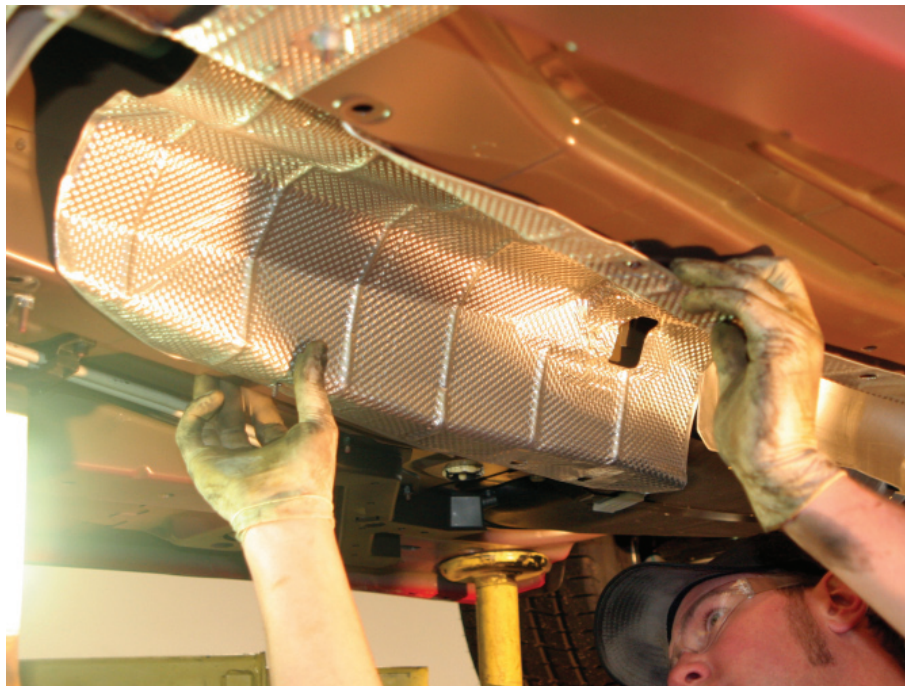
The heat shield was removed to access the driveshaft.
