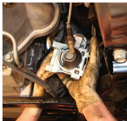
The starter motor must also be unbolted and set aside.
