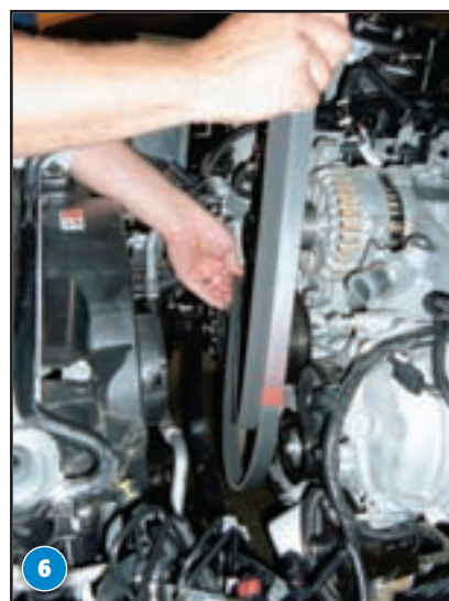
6 Loosen the belt tensioner and remove the stock belt.
